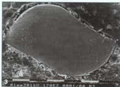
Figure 3: SEM image of Mtwo instrument cross-section, showing the two blade cutting surfaces resulting in an 'italic S' design
