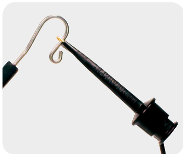
Stand-alone length determination with a hand file (without preparation)
